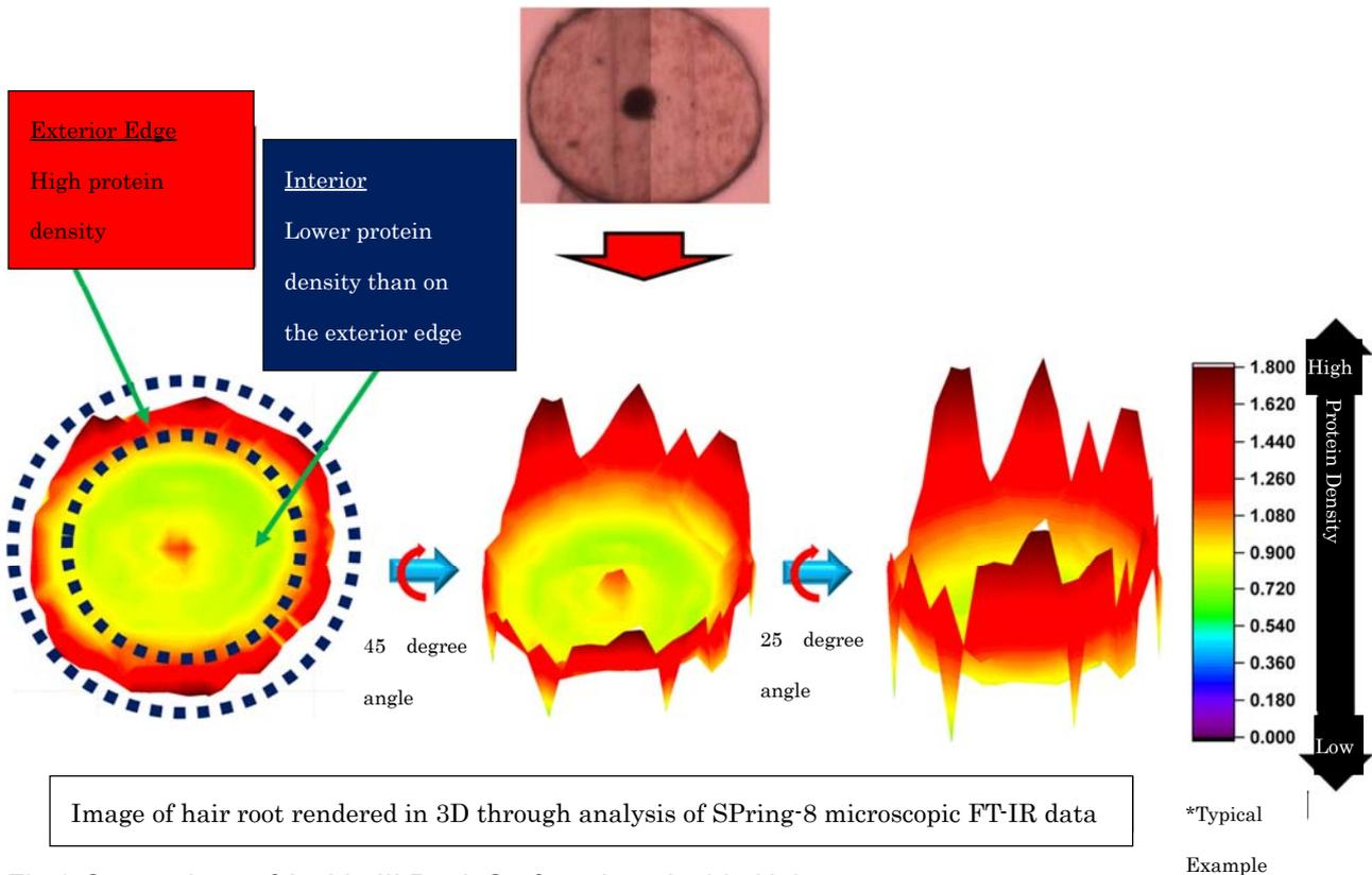
Fig.2 Comparison of Amide III Peak Surface Area Inside Hair
